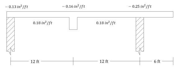
**Figure 7: Reinforcement Area Required**
