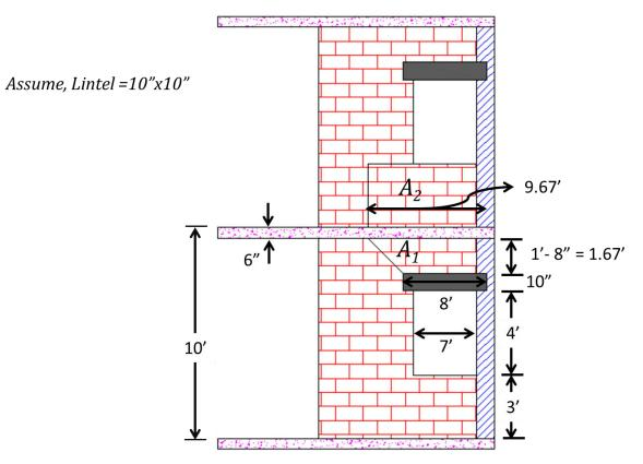
Figure 26: Information necessary to determine lintel load
