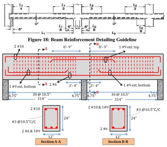
Figure 19: Beam Reinforcement Detailing According to the Design
