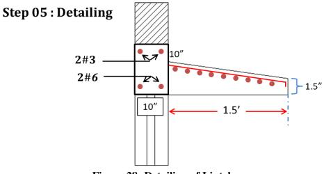
Figure 28: Detailing of Lintel
