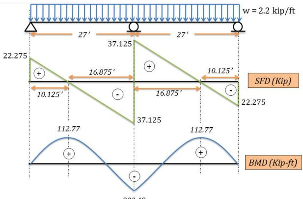
200.48 Figure 15: Shear Force Diagram and Bending Moment Diagram
