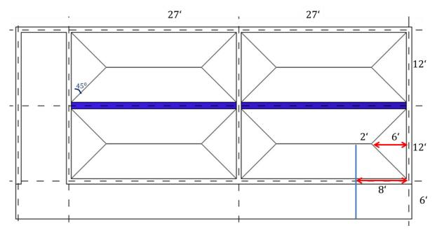
Figure 27: Loads come to Lintel from Slab
