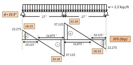
Figure 16: Shear Force Diagram of Beam
