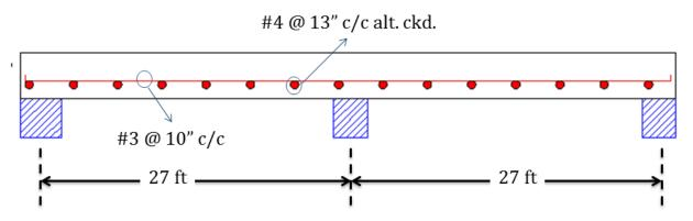
**Figure 10: Detailing at Section 2-2**
