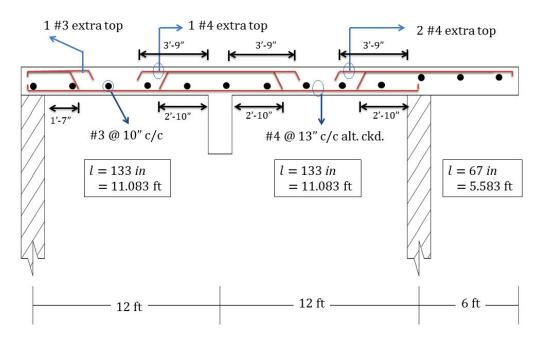
**Figure 9: Detailing at Section 1-1**
