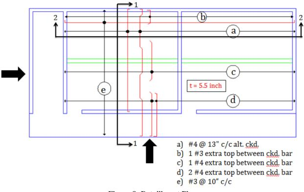
Figure 8: Detailing at Plan
