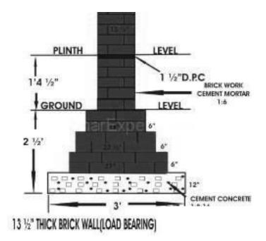
Figure 29: Typical Brick Foundation
