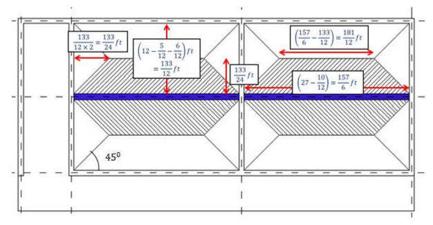
Figure 13: Determination of Contributing Area for Load Calculation
