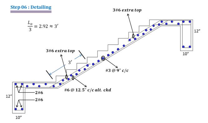
Figure 23: Reinforcement Details of stair.
