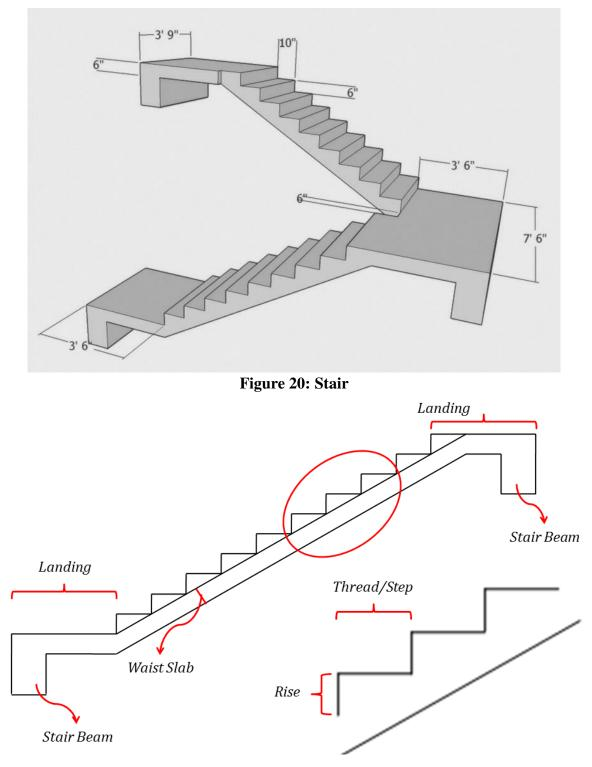
Figure 21: Components of Stair
