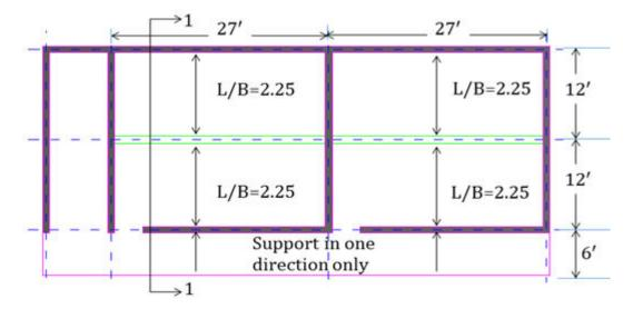
Figure 4: Load Transfer in Shorter Direction
