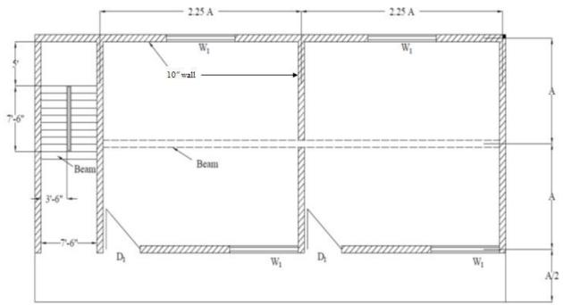
Figure 3: Typical Layout of Load Bearing Building
