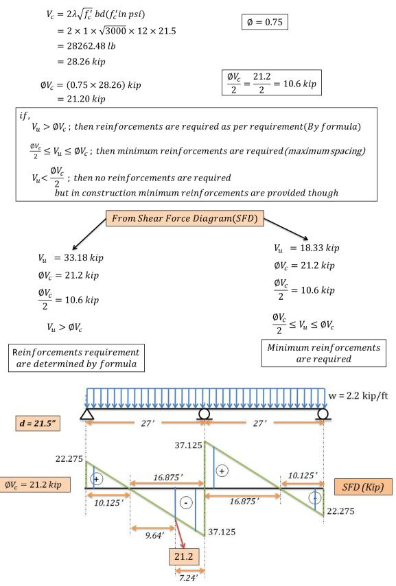
Figure 17: Distance determination where  $V_u = \emptyset V_c$
